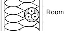
Room  | Multi-core cable direct in a thermally insulated wall <sup>a</sup>                                                                           | A1                                                                                            |
