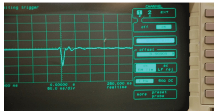
Figure 4 – Second discharge pulse that occurs as shown in Figure 2
