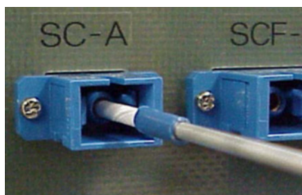
Figure 8 – Cleaning ports using a stick type cleaner
