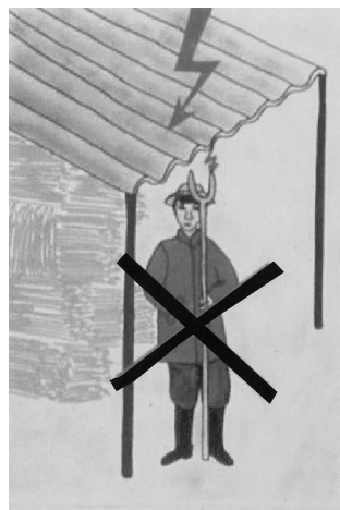
Figure 4 – Unsuitability of metallic structures when not earthed
