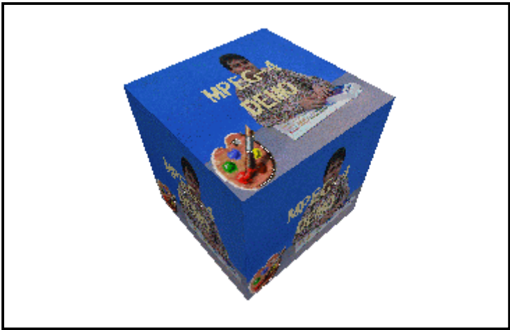
Figure 15 - A CompositeTexture2D example. The 2D scene is projected onto the 3D cube.
