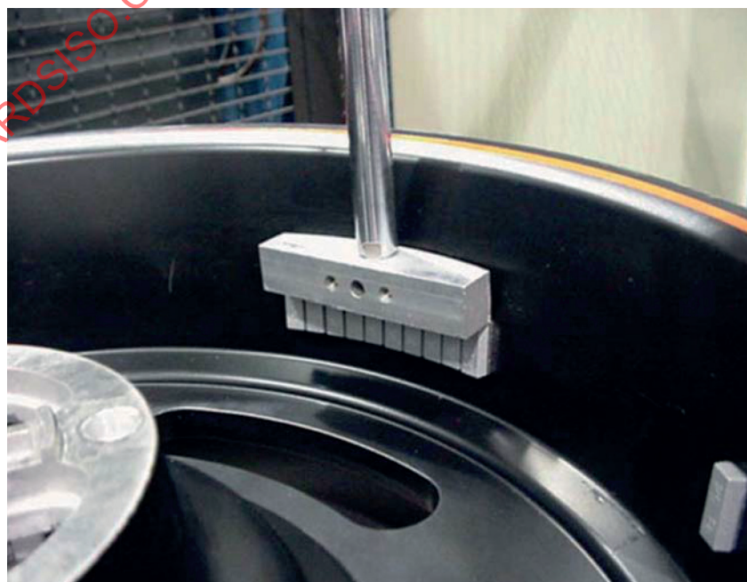
Figure 11 — Shear test method for adhesive weights
