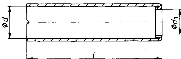
Figure 2 — Cylindrical tube with rolled-in end (type B)
