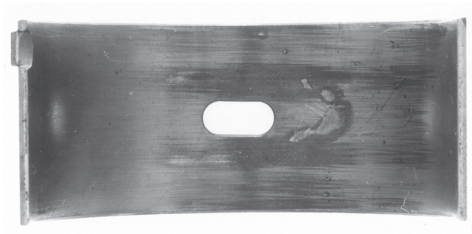
Figure 11 — Impact cavitation erosion near the end of an oil bleed slot in the rod half of a big-end bearing
