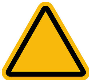
Figure 8 — Safety shape for warning signs
