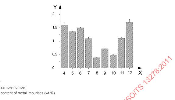
Figure A.3 — Total mass percentage of metal impurities in MWCNT samples provided by various manufacturers
