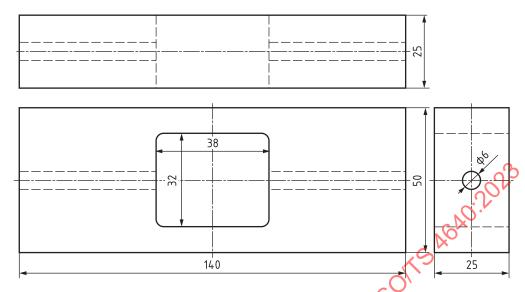
NOTE 3 The drawing on the top is a longitudinal section of the block, the one on the bottom is a top view, and the one to the right is a side view.
