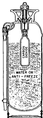
Figure D-4-1.6 Cartridge-operated Water Fire Extinguisher.
