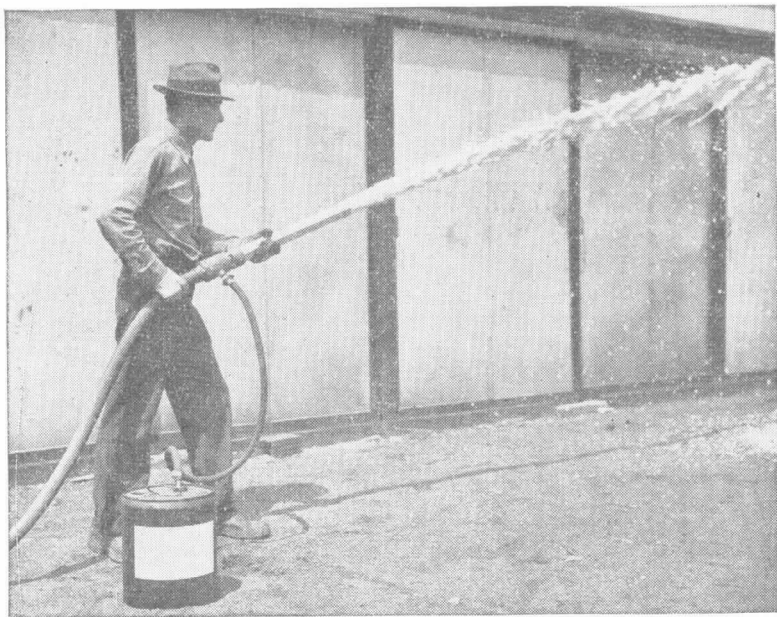
Fig. A-11-53. Air Foam Playpipe.
