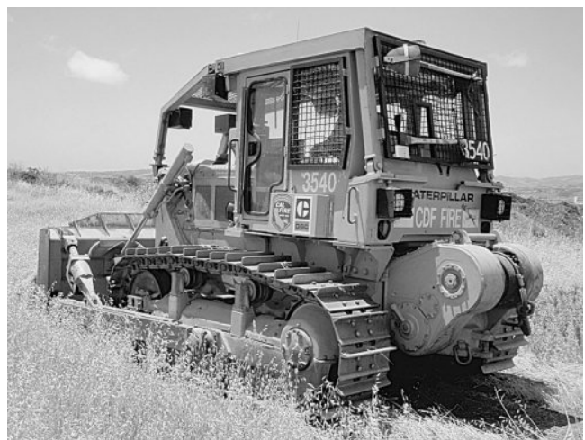
FIGURE A.5.1.3.2(3)(a) A Dozer Equipped with Protective Canopy, Lights, Brush Guards, and a Winch.
