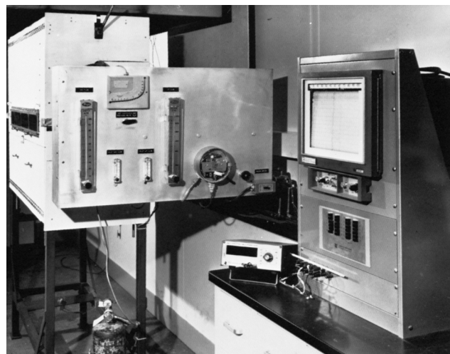
Figure 2-1(a) Flooring radiant panel test apparatus.
