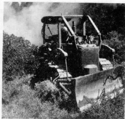
Tractor, angle dozer equipped and cable operated. Angle dozers may be positioned to operate as straight dozers. Brush guards are recommended for tractors which are to be used in the woods.
