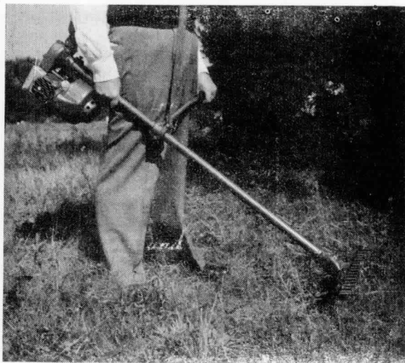
(Left) Typical shoulder-carried brush cutter which is useful for clearing fire line. These clearing machines are powered by two-cycle gasoline engines rated from 1\frac{1}{2} to about 3 horsepower.
