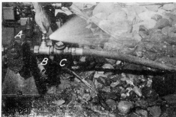
A indicates the pressure relief valve. C is a check valve. Its purpose is to hold the water in the hose line on slopes when the pump is stopped. Without it, water in the hose line would flow, by gravity, back toward the pump, causing it to turn in reverse as well as to lose all the water in the line. B is a hose tee with shutoff valve.
