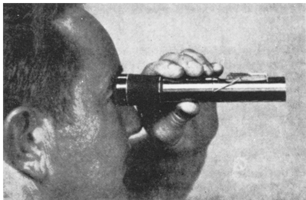
FIGURE A.6.2.2(b) Holding This Type of Refractometer Up to a Light Source to Take a Reading Where the Dark Field Intersects the Numbered Scale.
