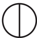
FIGURE A.16.3(c) Symbol that Represents Alternately Act as Start and Stop or On and Off — IEC Symbol Number 5010.
