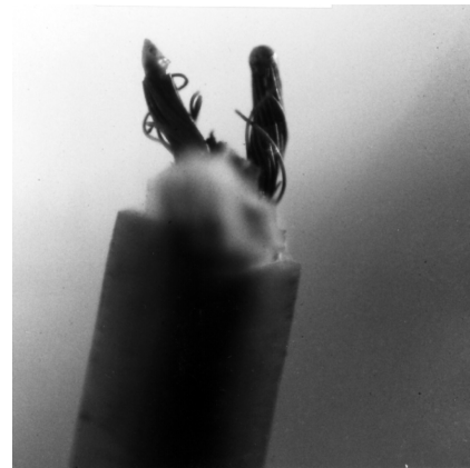
Figure 14-10.3(c) Stranded copper conductors severed by arcing through charred insulation with the strands terminated in beads.
