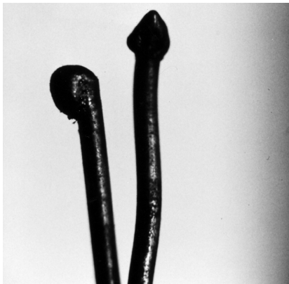
Figure 14-10.3(a) Copper conductors severed by arcing through the charred insulation.
