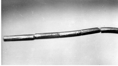
Figure 14-10.5 Aluminum conductor severed by overcurrent showing offsets.
