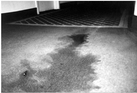
Figure 4-17.7.2 Irregularly shaped pattern on floor carpeting resulting from poured ignitable liquid. Burned match can be seen at lower left.
