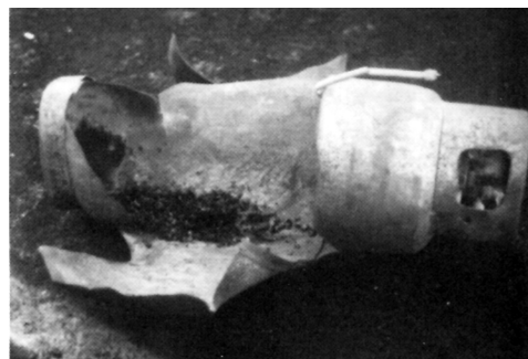
Figure 13-2.1.1(a) An LP-Gas cylinder that suffered a BLEVE as a result of exposure to an external fire.
