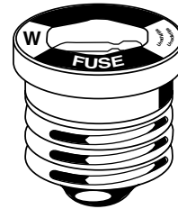
Figure 14-6.1(a) A typical, Edison-based nonrenewable fuse, single element. For replacement purposes only.
