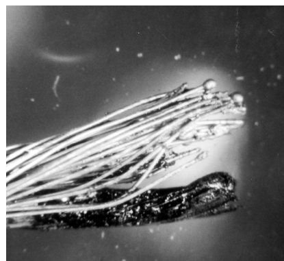
Figure 14-10.2(b) Stranded copper lamp cord that was severed by a short circuit.
