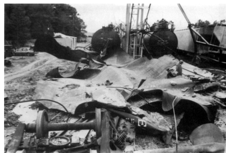
Figure 13-2.1.1(b) A railroad tank car of butadiene that suffered a BLEVE as a result of heating created by an internal chemical reaction.
