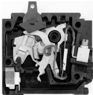
Figure 14-6.2(c) A 15-A residential-type circuit breaker in the open (tripped) position.
