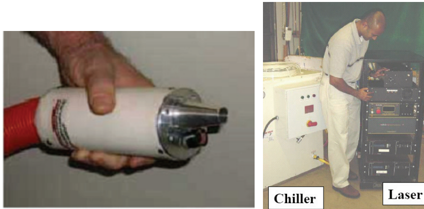
FIGURE 7 - GENERAL LASERTRONICS END EFFECTER/ LASER SYSTEM AND CHILLER
